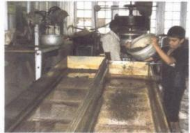
Roll breaking is done to separate well twisted fine bulk from untwisted big bulk which is to be charged for next rolling. Here small particles will pass through mesh and big bulk will go for next rolling
