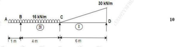
Q.4 (a) A continuous beam ABCD is loaded as shown. The support B sink by 10 mm. Draw BMD, Use moment distribution method. Take E =200 X 10<sup>6</sup> kN/m<sup>2</sup> and I = 100 X 10<sup>6</sup> mm<sup>4</sup>
