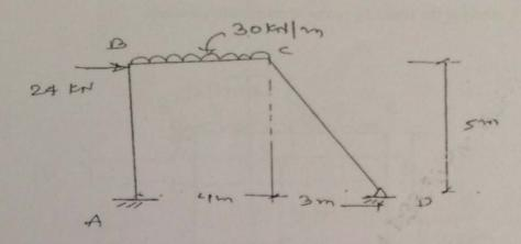
4. (a) Analyse frame by slope defection method and draw B.M.D
