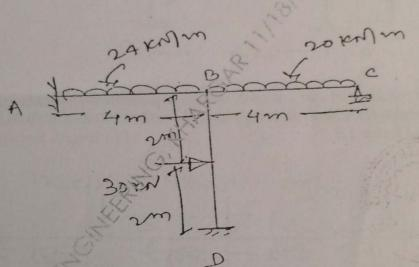
(b) Analyse the beam by three moment theorem and Draw B.M.D
