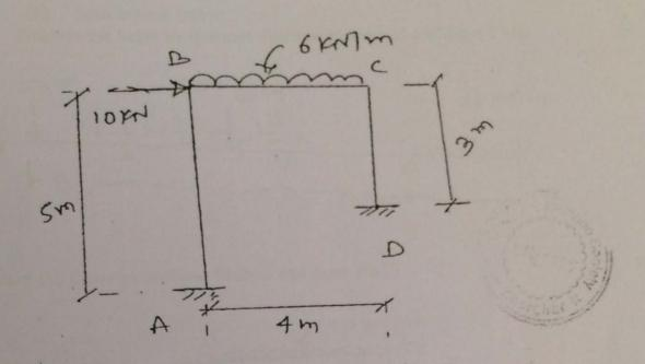
3. Analyse the frame as shown in fig by slope deflection method and draw BMD.
