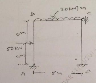
(b) Determine the plastic moment capacity for the bean as shown in fig. lake Load factor 1.5
