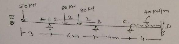
5. Analyse the frame by stiffness method and draw BMD.
