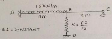
Q.3 Analyze the rigid jointed plane frame using Flexibility Method. Also draw BMD and deflected shape of the frame. Take EI = Constant for all members. (20)
