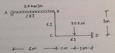
Q.7 Analyze the continuous beam loaded and supported as shown in figure using Moment Distribution Method. Also draw SFD, BMD and deflected shape. Note that the supports at 'B' settle by 10 mm. Take EI = 20000 KNm<sup>2</sup>. (20)
