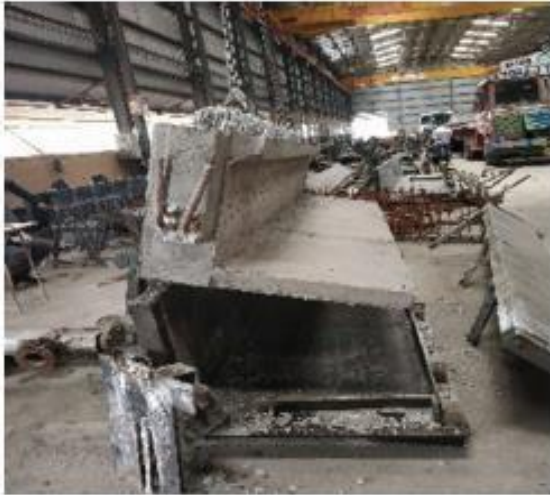
Figure 3. Chajja Beam capacity of the beam unit is 165 beams per day.
