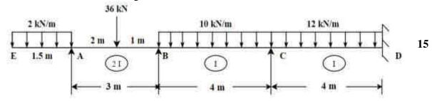
Q.3 (a) Find the Plastic Moment 'Mp' for the continuous beam given below.
