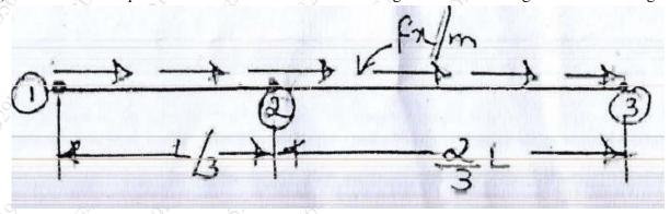
**b)** Assemble the equation of equilibrium for a spring system as shown as shown in Figure by direct approach. Show that minimization of Potential of Potential Energy also yields the same result (stiffness method)
