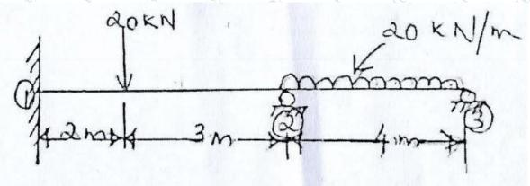
3. a) Determine the equivalent nodal loads due to udl of magnitude fx/unit length as shown in figure 10
